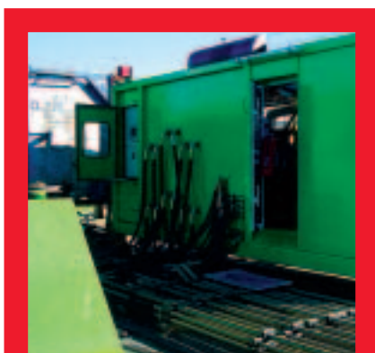
IHC Hytop's hydraulic power pack and piping
