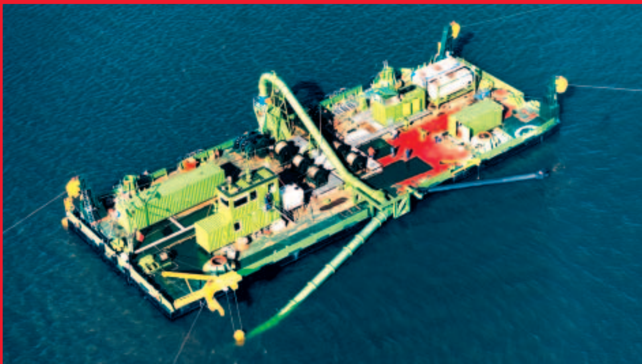
Gravel spraying pontoon BAYARD II, owned by Dredging International
