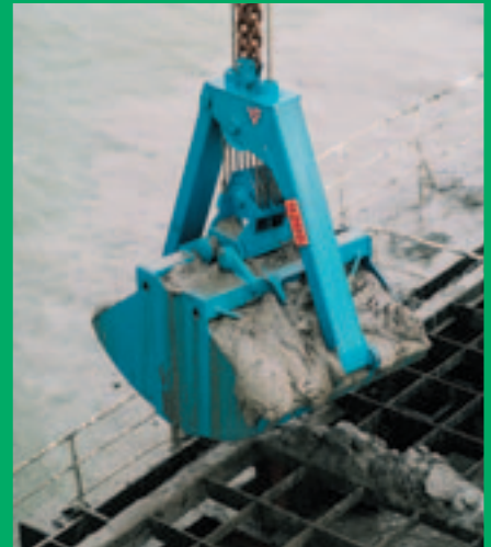
The 2m 3 grab during dredging trials
